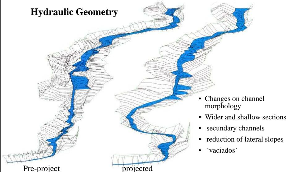
Study hydraulic conditions from topographic cross sections (pre-project) and from designed ones (HEC-RAS).
